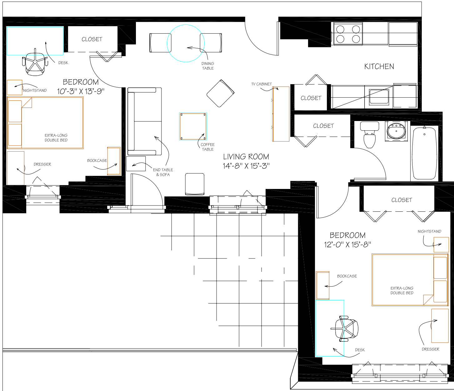
TYPE 13 Typical Apartment - 2 Bedroom - 720 sq.ft. Locations: 6J 1 apt. Total # Type 13 apts. 1 apt.
