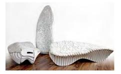
The future of furniture may be in building materials made from biological matter. Mycoform, a product combining a type of fungus with precise compacted forms of inert waste (such as discarded wood chips, oat bran, and gypsum), is the basis for these prototypes from Terreform ONE and Genspace.
